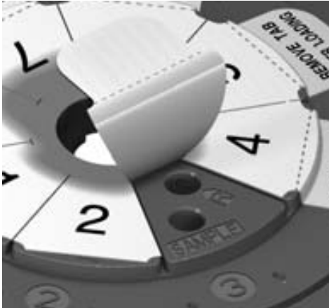
Figure 1 - Disc with pre-use foil lifted from Sample and Reaction Wells for wedge #3
